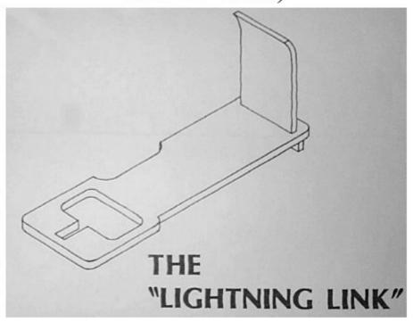
The parts for the Lightning Link can be made from tool steel, machined with great precision, hardened and tempered with loving care, the polished to a high gloss that your mother would be proud of. On the other hand, using only a couple of pieces of power hacksaw blade to make the parts from, a dremel tool, hand drill and one or two files to do the work, you can cut out the Lightning Link in about an hour.
